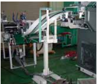
Product infeed includes crusher rolls, controlled gapping mechanism, product divert, and inverting spiral conveyor. A wide variety of equipment arrangements may be accommodated.
