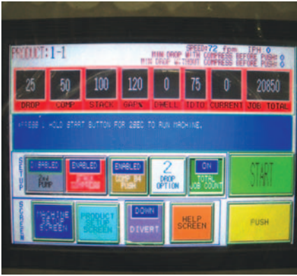
Simplified operator controls utilizes fewer adjustment knobs and displays numeric indicators. Prior job settings are saved and recalled for the next job run.
