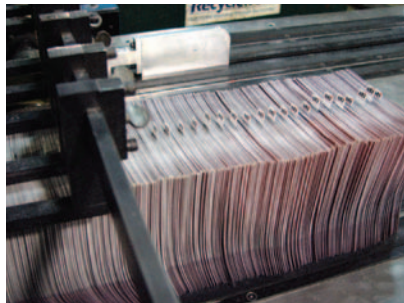
Tabs act as flags to locate the start and finish of the exact count
