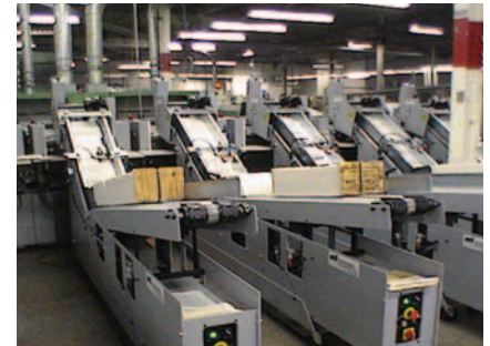
SuperFeeder-XA is available in a version that has an adjustable angle on the load conveyor to best suit the products being run.
